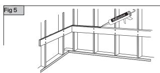
Apply construction adhesive to top of support strips.
